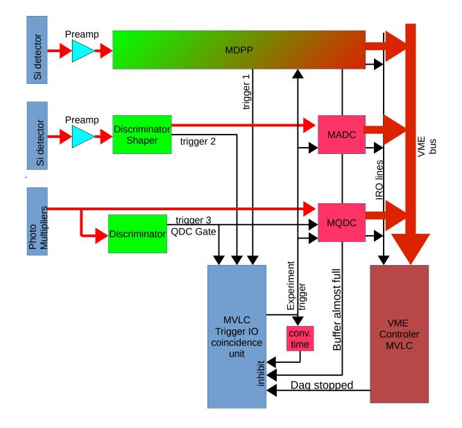
In the readout cycle it is also possible to read a fixed number of events per module. This increases the amount of data read in one cycle, and reduces the time overhead for handling interrupts.
