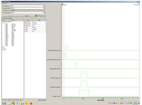
The following picture shows the 3 input signals at the top, followed by the 3 delayed and widened signals after passing the gate generators.
