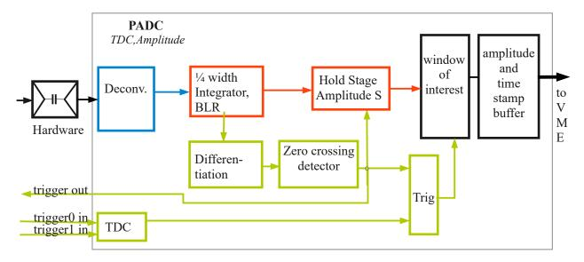
The signal is amplified filtered digitized. Then the pre-differentiation is removed by a deconvolution. Then the signal is integrated with a time constant of about ½ of the FWHW of the signal. This improves the resolution to up to 1/32000 of the full range.
