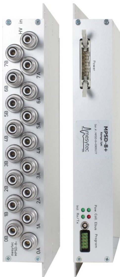
MPD-8+ in a stand alone box with fixture latches. Mechanical properties are identical to MSTD-16.
